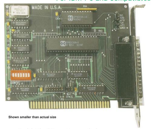
The CIO-DIO24/CTR3 combines digital input/output and counters on one board. It has the digital lines common to the PIO-12, PIO-24 and CIO-DIO24 boards, and is also connector compatible with them.
